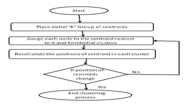
Figure 3: The Flow Chart for the k-means algorithm
