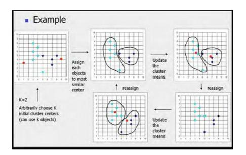
Figure 2: Original K-means Algorithm
